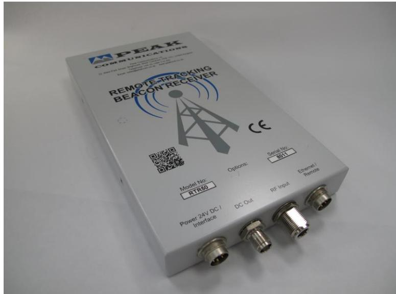
The **RTR50** is a next generation remote mounted tracking receiver, designed specifically to track and measure 'CW' beacons from commercial satellites. Primarily an L-Band input receiver, the unit is designed to be used for telemetry and control, typically in earth stations using medium to large antennae or for smaller antenna in typically SOTM applications.
