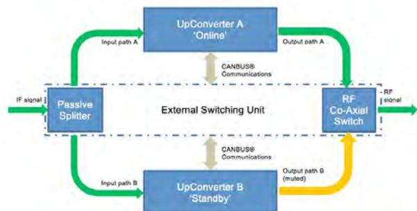
Fig.2: 1-for-1 Redundant Upconverter System with External Switching Unit
