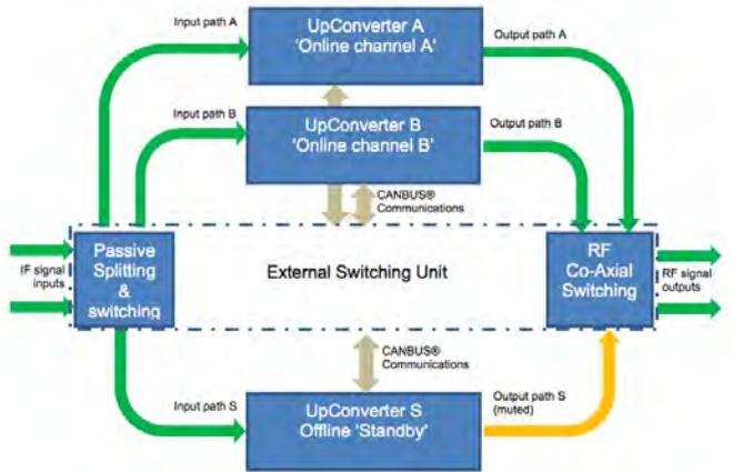
**Fig.4: 2-for-1 Redundancy UpConverter System with External Switching Unit**
