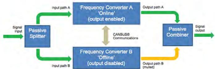
Fig.1: 1-for-1 Passive Redundancy
