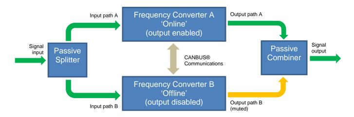
Both converters operate continuously, performing their conversion function on the incoming signals, but only one unit enables its output.
