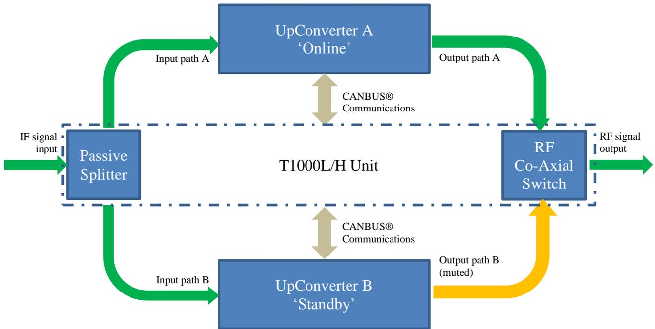
**P7xxx series UpConverter in 1+1 redundancy using T1000L/H**
