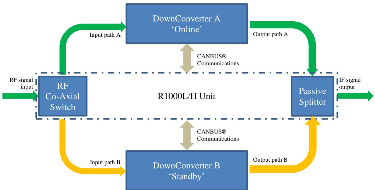
**P7xxx series DownConverter in 1+1 redundancy using R1000L/H**
